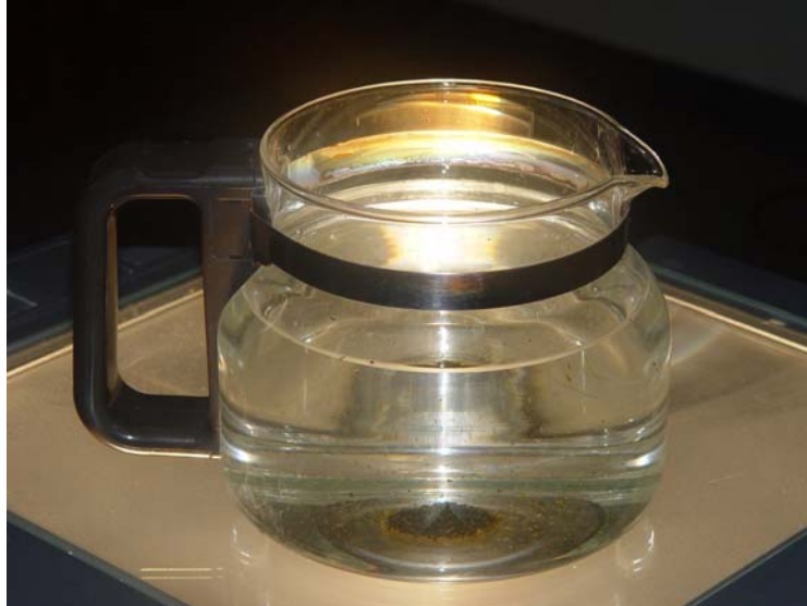
Figure 4.1: The beaker experiment showing the effects of frictionally-induced inflow near the bottom after the water has been stirred to produce rotation. This inflow carries tea leaves to form a neat pile near the axis of rotation.
