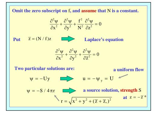
Streamfunction equation is linear
