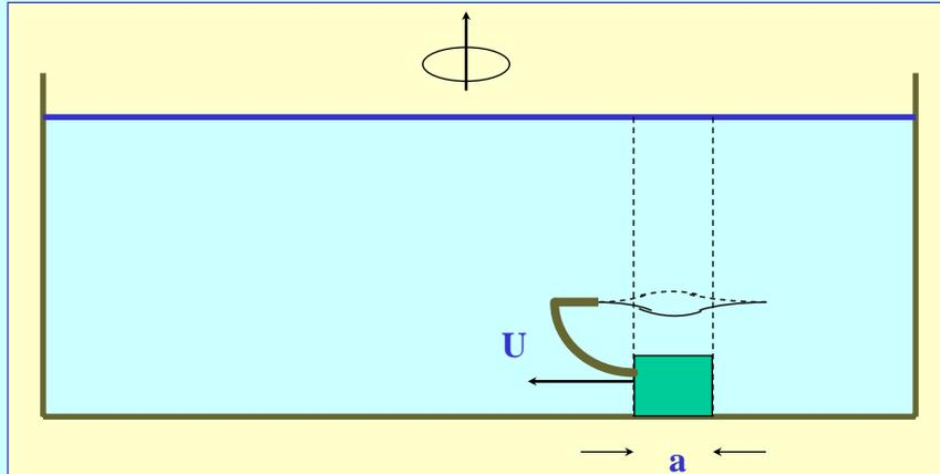
An obstacle with linear dimension  $a$  is towed with speed  $U$  along the bottom of a tank of fluid of depth greater than  $a$  in solid body rotation with angular velocity  $\Omega$ .
