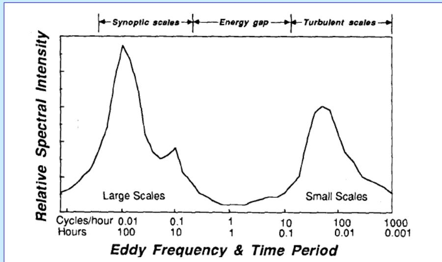
Schematic spectrum of wind speed near the ground.
