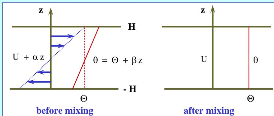
Before and after states in the complete mixing of a uniform shear layer with a uniform potential-temperature gradient.
