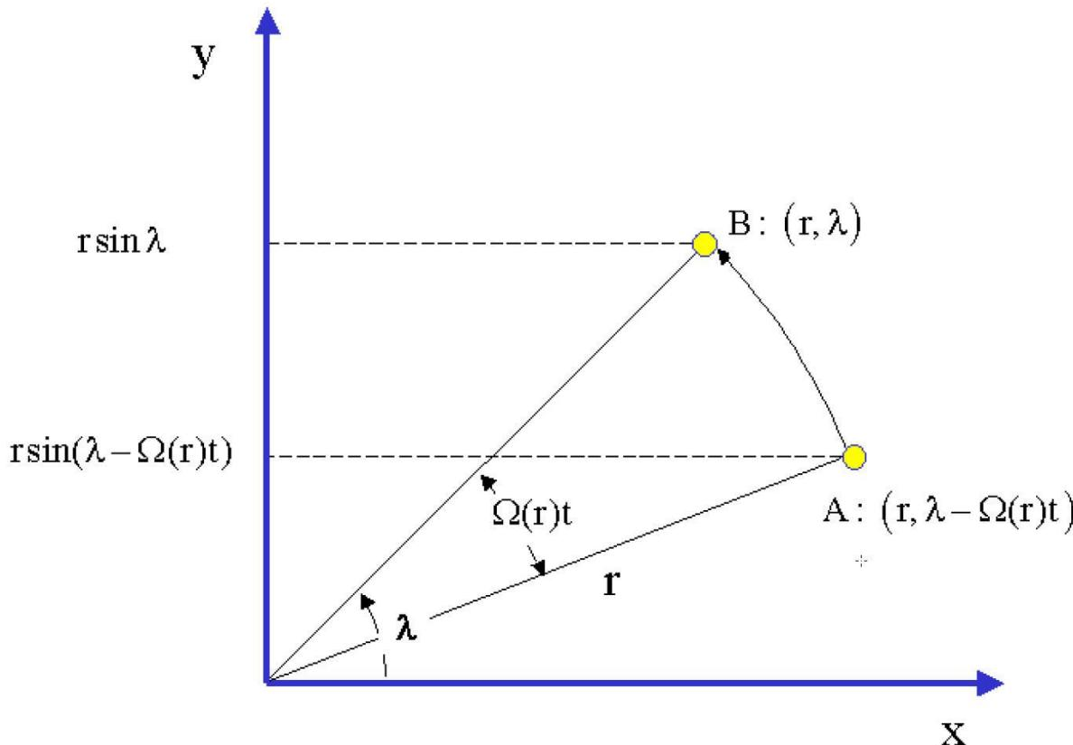
Figure 1.2: An air parcel moving in a circular orbit of radius  $r$  with angular velocity  $\Omega(r)$  is located at the point B with polar coordinates  $(r, \lambda)$  at time  $t$ . At time  $t = 0$  the parcel was located at point A with coordinates  $(r, \lambda - \Omega(r)t)$ . During this time it undergoes a meridional displacement  $r[\sin \lambda - \sin(\lambda - \Omega(r)t)]$ .
