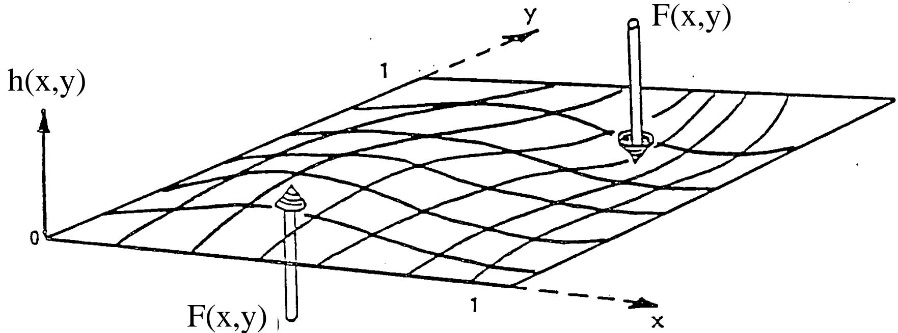
**Equilibrium displacement of a stretched membrane over a square under the force distribution  $F(x, y)$ .**
