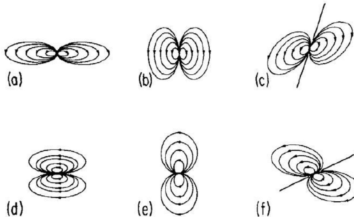
Figure 3.11: Streamfunction responses to point sources of: (a) Heat in a barotropic vortex with weak inertial stability, (b) heat in a barotropic vortex with strong inertial stability, (c) heat in a baroclinic vortex, (d) momentum in a barotropic vortex with weak inertial stability, (e) momentum in a barotropic vortex with strong inertial stability, and (f) momentum in a baroclinic vortex. (Based on Figs. 8, 9, 11, and 12)
