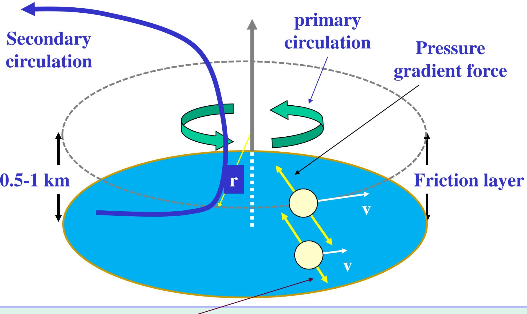
Centrifugal force and Coriolis force are reduced by friction
