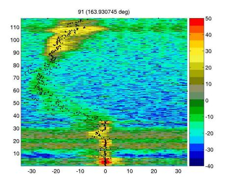
Figure 2: Waterfall plot taken of the radial at  $164^{\circ}$  from data taken on April 5, 2003 at KOUN. The *x*-axis corresponds to radial velocity (*m*/*sec*) and the *y*-axis to range (*km*) from radar. The color corresponds to the range-adjusted power of the power spectrum at that velocity (Doppler frequency) and range. The dots represent the mean velocity as computed by an algorithm, in this case the pulse-pair estimator.
