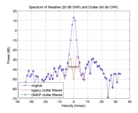
Figure 1: Simulated spectrum of a 20 dB signal to noise ratio weather spectrum centered at 15 m/sec with a 60 dB clutter to noise ratio clutter spectrum centered at 0 m/sec. The original spectrum in shown in blue, the spectrum after the high suppression legacy clutter filter is shown in red, and the spectrum after a high suppression GMAP filter is shown in black. Within the green circle is the clutter power residual after clutter filtering.
