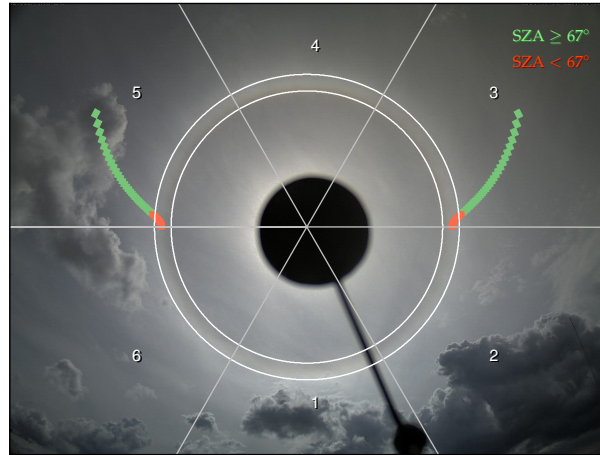
Abbildung 4.7: HaloCam image as in Fig. 3.20b. The red and green squares indicate the minimum scattering angle of the sundogs as a function of the solar zenith angle (SZA). The SZA ranges between 90^\circ and 35^\circ with 1^\circ resolution. The mask used to search for the 22^\circ halo peak is displayed by the two white circles and covers scattering angles between 21.0^\circ and 23.5^\circ . Sundog positions located within this mask might be mis-classified as 22^\circ halo and are marked as red. These positions correspond with SZAs between 90^\circ and 67^\circ . For smaller SZAs (higher solar elevations) the sundogs are located outside the mask and cannot be mis-classified as 22^\circ halo by the algorithm.
