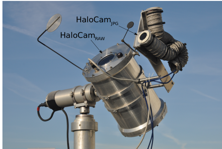
Abbildung 3.17: HaloCam-setup with different wide-angle cameras: \text{HaloCam}_{\text{JPG}} represents the Mobotix S14D camera model which consists of one camera body and two lenses with 4 mm focal length. One lens is centered relative to the sun, the other lens is pointing to the zenith and is not used for this study. This camera records pictures only in the compressed JPEG format. \text{HaloCam}_{\text{RAW}} represents the Allied Vision Manta G-235 C camera model with a Kowa wide-angle lens with 6 mm focal length, which provides the uncompressed “raw” signal measured at the sensor.
