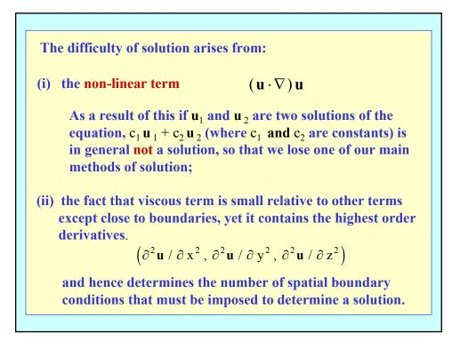
The Navier-Stokes equation is too difficult for us to handle at present and we shall concentrate on Euler's equation from which we can learn much about fluid flow.
