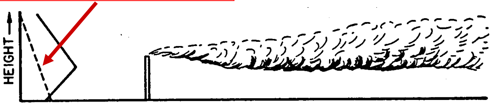
TEMPERATURE INVERSION BELOW, LAPSE ALOFT (LOFTING)
