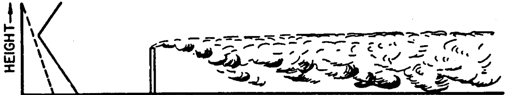
TEMPERATURE LAPSE BELOW, INVERSION ALOFT (FUMIGATION)
