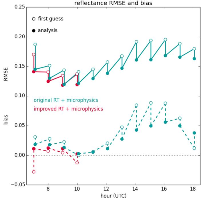
Evolution of the reflectance RMSE and bias of the ensemble mean for different assimilation experiments started at 18 June 2012, 12UTC. Left: Runs with SEVIRI and/or conventional observation and an assimilation interval of 3 hours. Right: Runs with original and improved RT and microphysics settings and an assimilation interval of 1 hours.
