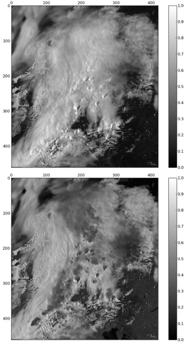
FIG. 3. Reflectance simulated with the 3D solver MYSTIC at 15 UTC on June 22nd 2011 (SZA=50°). The central wavelengths used are 635 nm corresponding to the SEVIRI channel VIS006 (upper plot) and 1.64  $\mu\text{m}$  corresponding to the SEVIRI channel NIR016 (lower plot).
